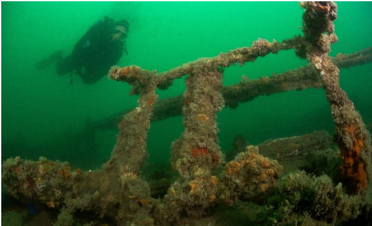
Figure 4: The portside nacelle which would have housed the V12 engine. Photo: Matt Doggett.
