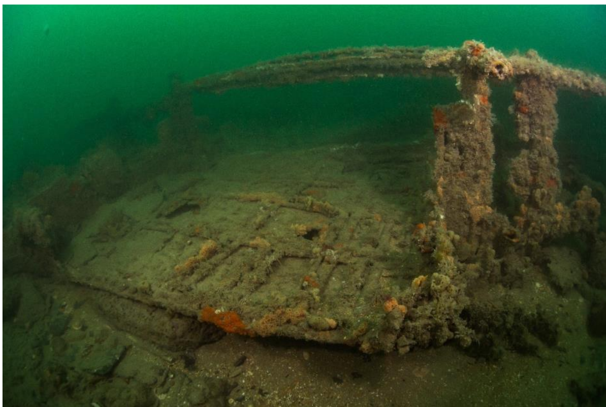
Figure 17: The lattice framework in the wing structures was where the forward and rear fuel tanks were housed. The nacelles which supported the engines are visible on the right. Photo: Matt Doggett.
