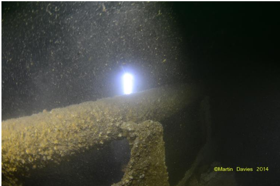
Figures 10 and 11. Propeller shaft showing the shaft, flanges and thrust block and bearings
