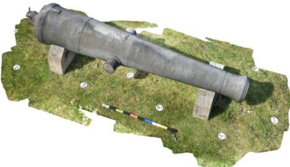
Figure 6 use of photogrammetry targets and scale (© Martin Davies)
