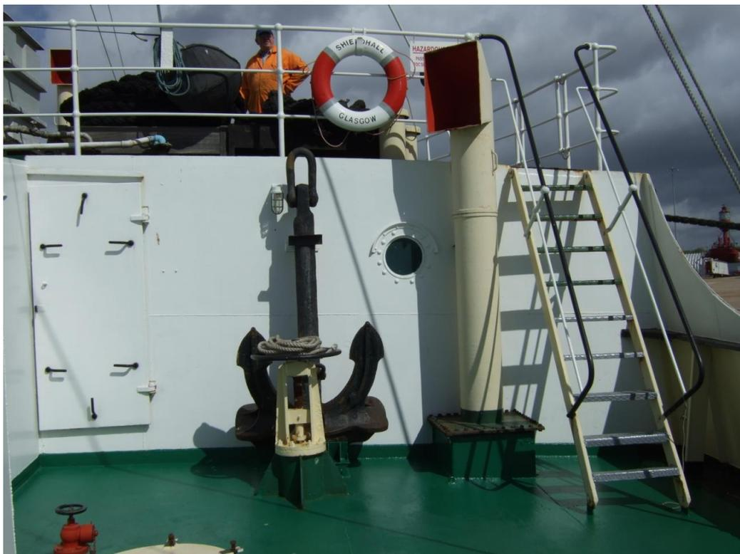
Figure 34. Spare anchor and top of a ventilation shaft. Photograph Jane Maddocks
