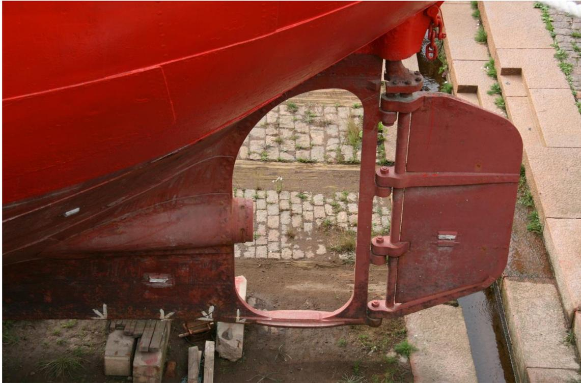
Figure 39. Stern assembly showing rudder, fixings and propeller shaft. Photograph. Jane Maddocks.
