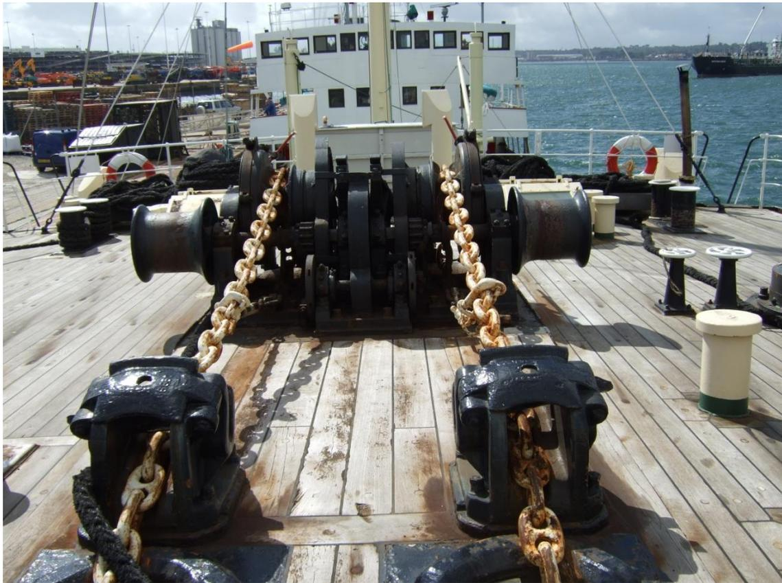
Figure 32. Anchor winches showing machinery and chain. Photo© Jane Maddocks by kind permission of the SS Shieldhall management team.
