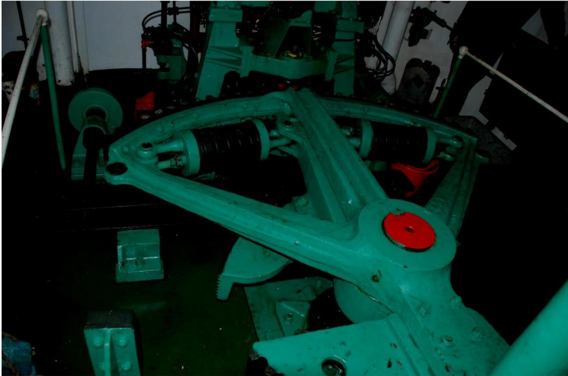
Figure 37. Steering arc for rudder control. Photo Jane Maddocks by kind permission of SS Shieldhall management team.
