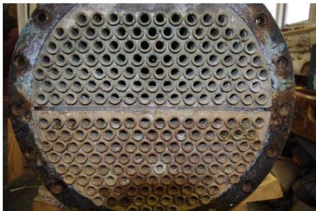
Figure 43. Condenser from Pinnace 199 ©Steam Pinnace 199 group.
