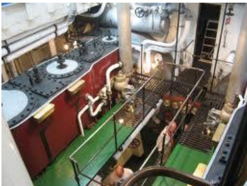
Figure 44. Top of a triple expansion engine, showing three cylinders. Reproduced by kind permission of the management team from SS Shieldhall.
