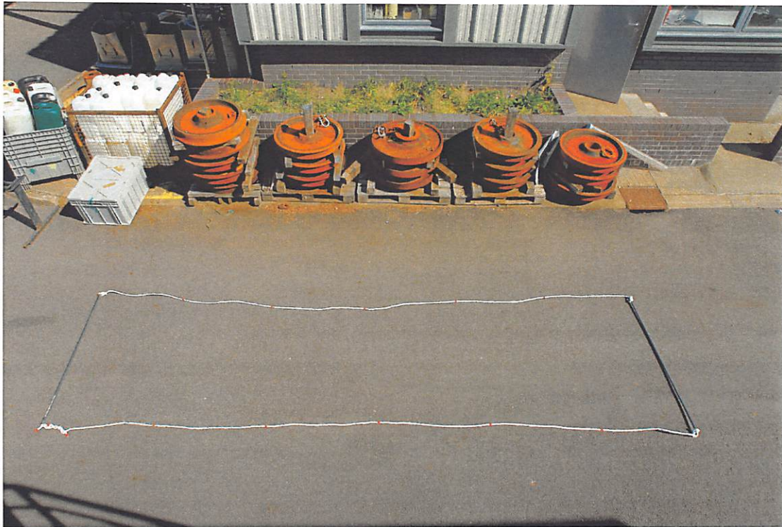
Fig 2.1 Belt Transect prior to deployment. The transect would be rolled up in the manner of a scroll and thus could be deployed with ease by a team of two divers working together.
