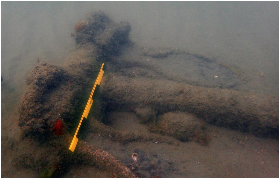
Figure 28: Large stockless anchor, probably a relic from World War II training exercises in Bracklesham Bay associated with Exercise Fabius III.
