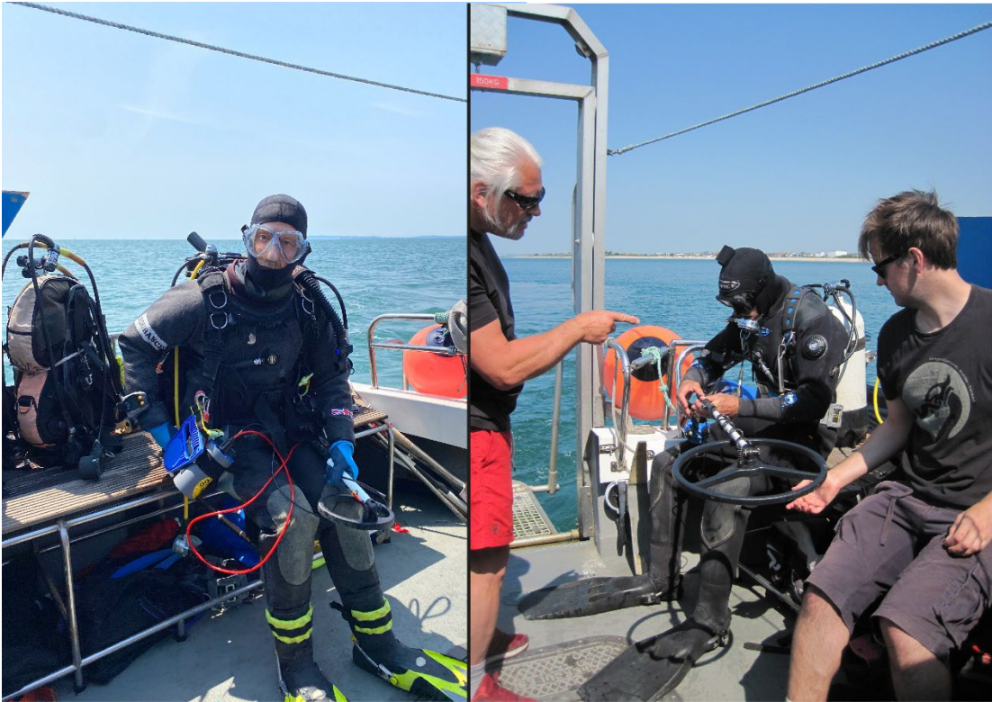
Figure 25: Divers with Aqua Scan metal detectors. Diver on left has the smaller 8 in search loop and the diver on the right has the larger 15 in search loop.
