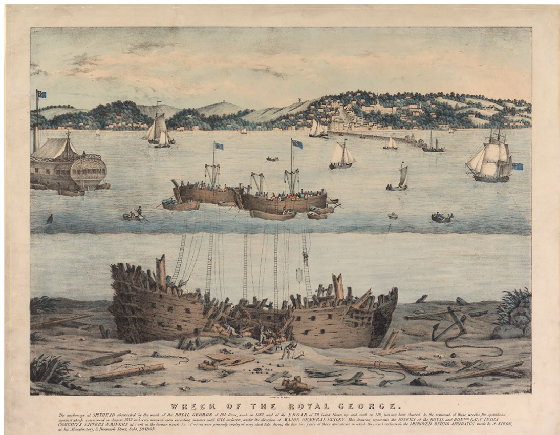
Figure 4: Shows two slave vessels over the wreck of Royal George with lifting gear. Alongside these vessels are two smaller boats which could represent the lighters carrying the dive pumps and explosives. These vessels match those used on Edgar . Also note in the background, the town of Ryde and it's pier on the Isle of Wight.
