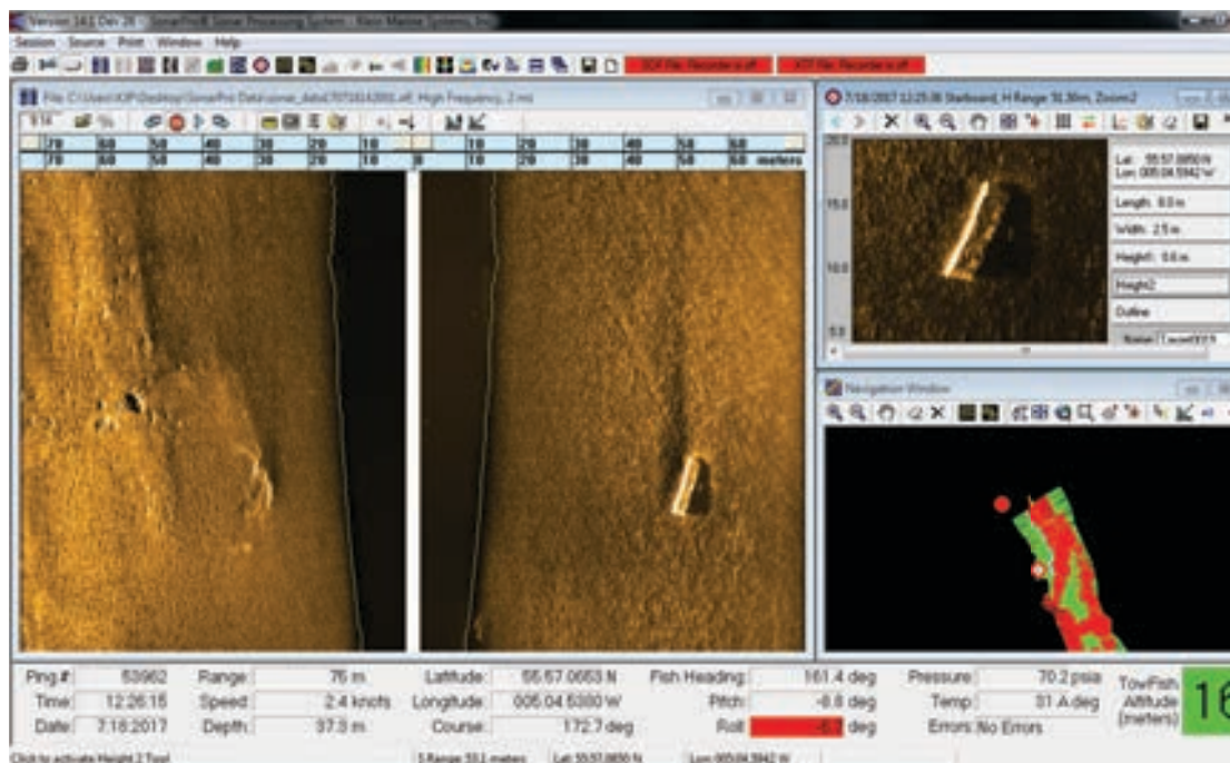
Fig 9: Side-scan of discovered isolated X craft side charge
