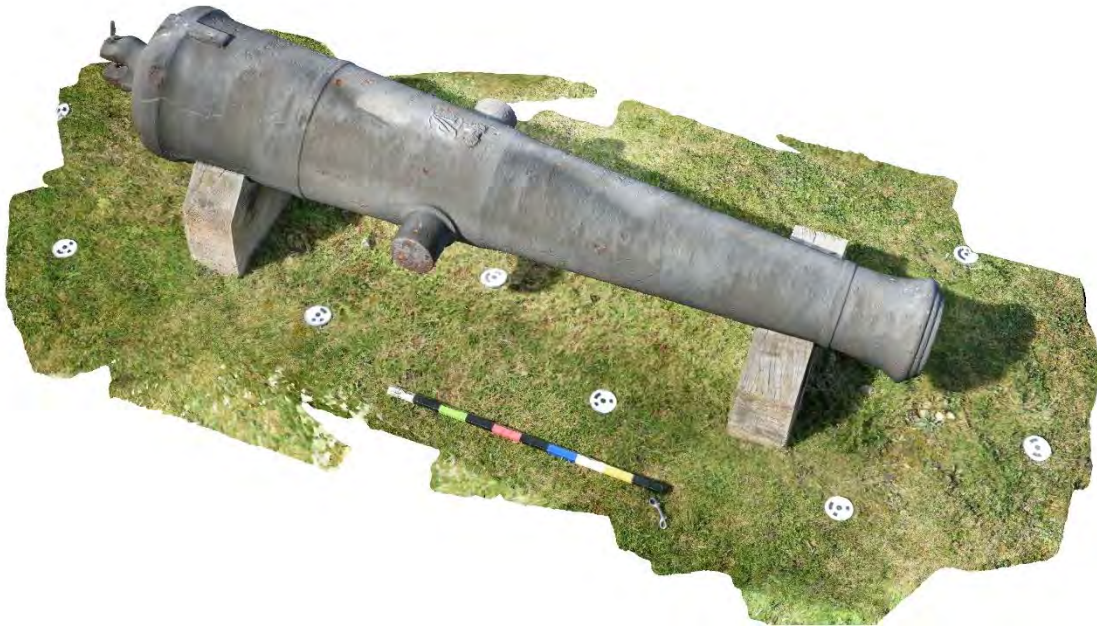
Figure 5 use of photogrammetry targets and scale (©Martin Davies)
