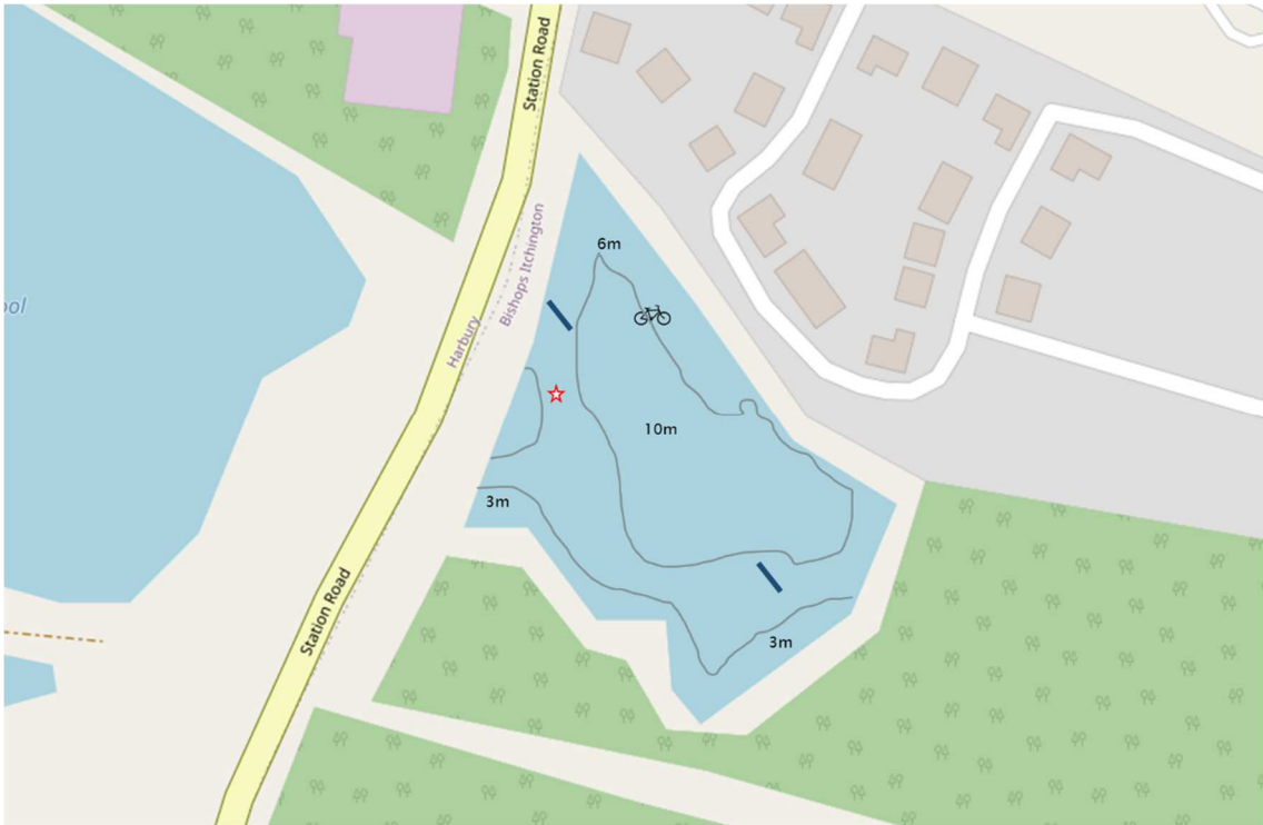
Figure 50 Sketch map of Blue Pool based on diver observations and bathymetry showing the remains of iron rails (blue lines). The location of the monitoring station is marked by a red star. [31]
