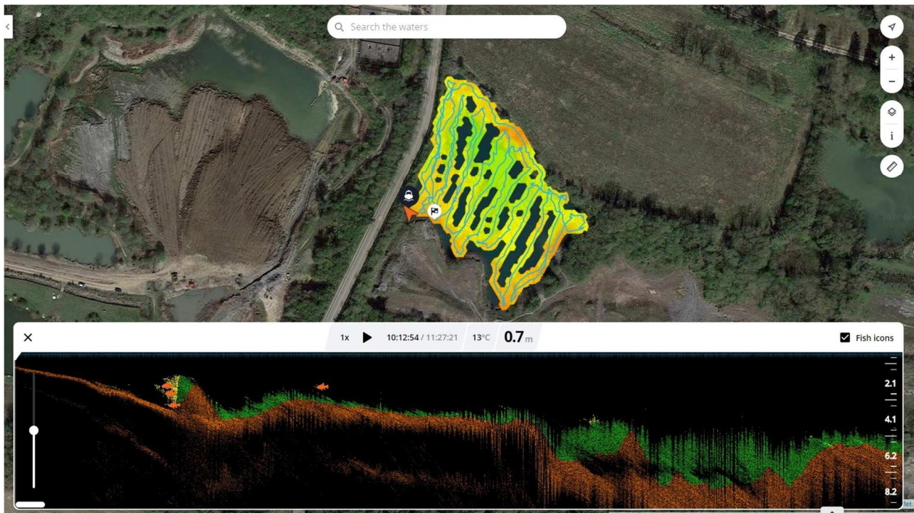
Figure 36 Blue Pool bathymetry data showing the route of the kayak across the water (blue line overlaying the map) and a depth profile (insert below).
