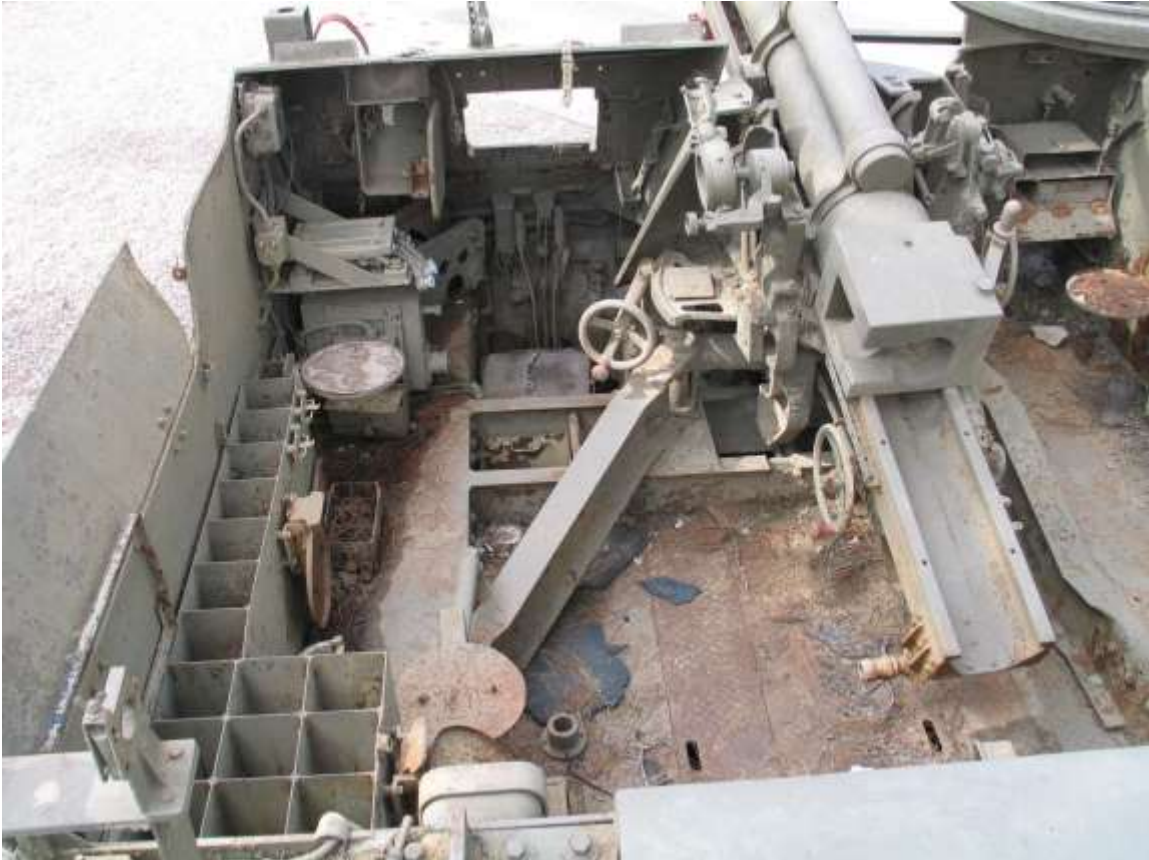
Figure 47 M7 Howitzer 105mm self-propelled gun (© Tom Templeton)
