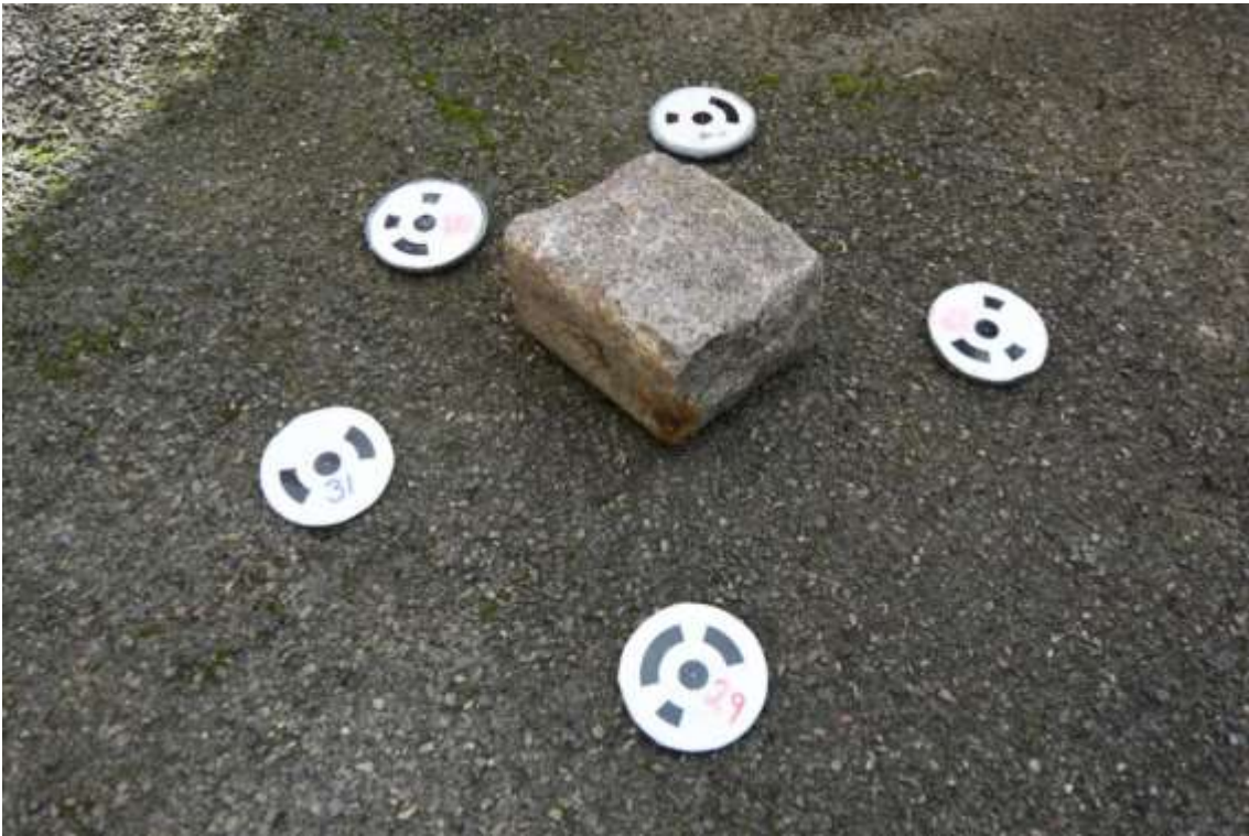
Figure 4 Use of photogrammetry targets (© Martin Davies)
