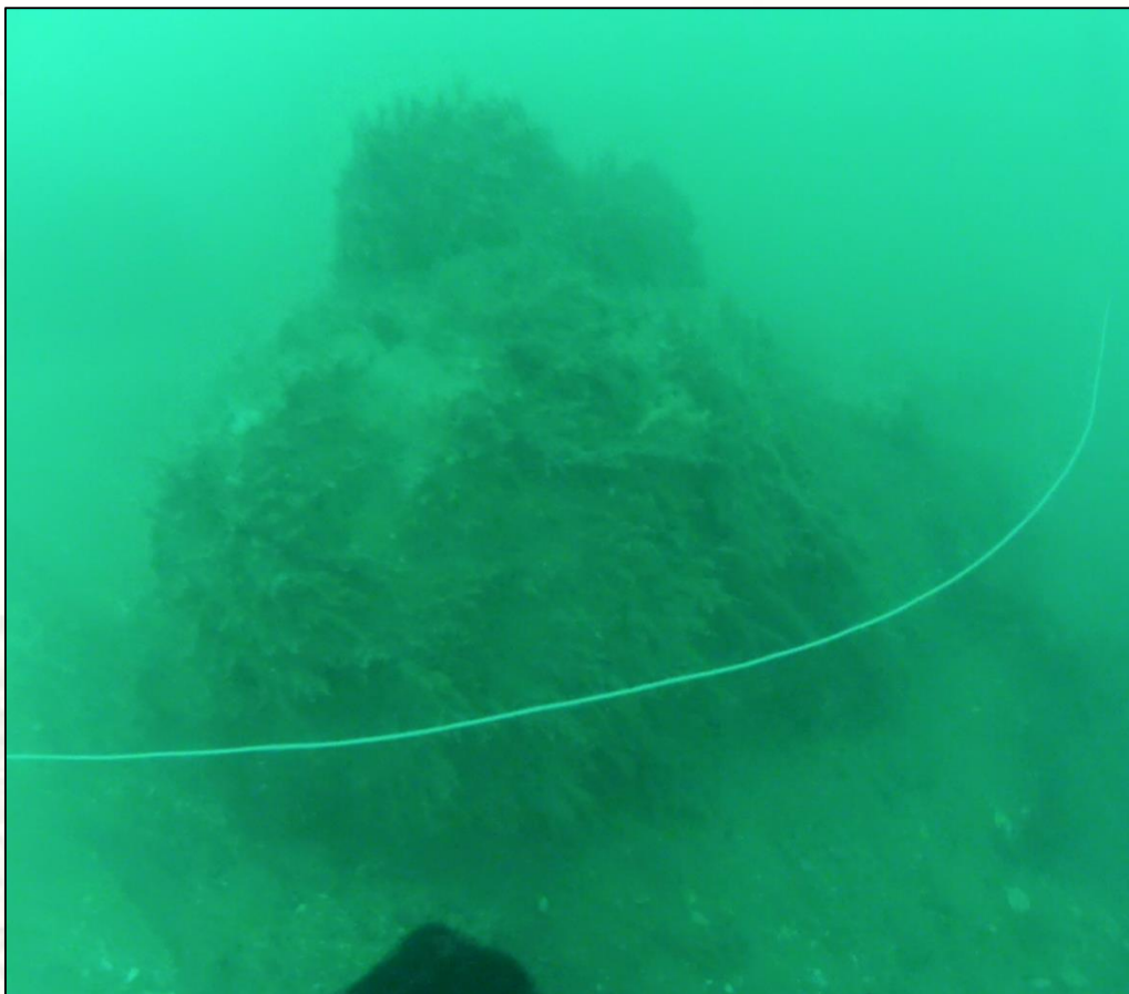
Figure 19 Stem post and bow area showing heavy weed growth, possibly due to fishing gear snag.
