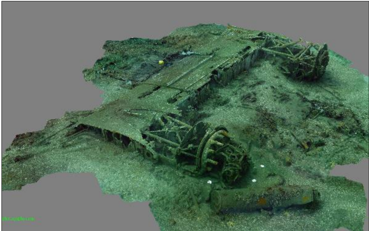
Figure 25 Side view of C-47 taken from the 3D photogrammetry. Note the possible Mark V mine in the foreground, starboard engine hanging off its mount and large debris field between the two engine mounts.
