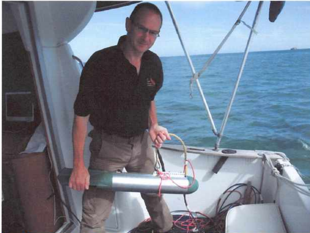
Figure 2 Diving Officer Martin Davies launching the side-scan sonar 'fish' (Image Alison Mayor)
