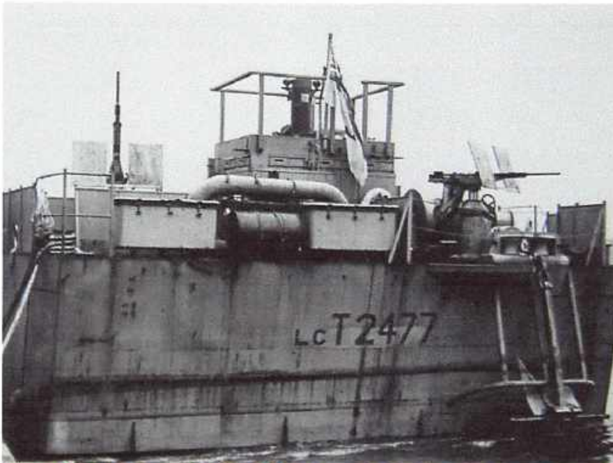
Figure 11 - The stern of LCT 2477 showing 2x Oerlikon 20mm anti-aircraft guns. Note also the large keedge anchor.
