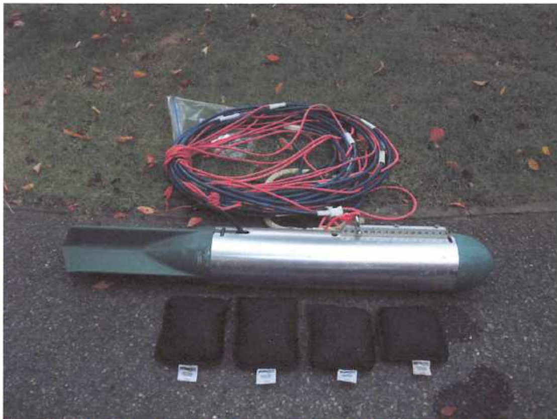
Figure 1 -Side Scan Sonar equipment kindly loaned by Nautical Archaeology Society (NAS)
