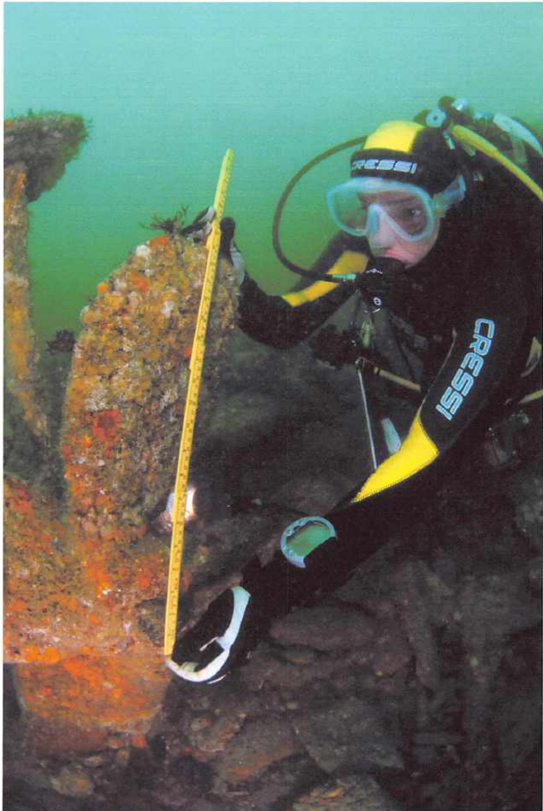
Figure 11 - Propeller - 4 blade and 37 inch diameter (Image Martin Davies)
