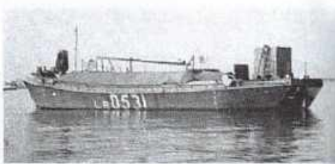
Above: An LBR fitted with a stern ramp and steering position aft and armed with an MG. forward. (J.W.A.)
