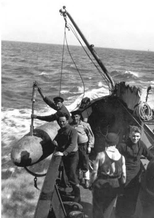
Steaming the starboard sweeping gear. The cutting gear to sever the mooring cable of high explosive mines is supported by an Oropesa float, seen here swung out on a davit.
