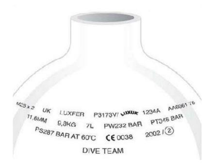
12. A cylinder has the above markings. What is its buoyancy in fresh water when empty? State your answer to the nearest kg (You should assume that density of aluminium is 2,600 kg / m³, and that the valve has a mass of 200g and of negligible volume)
