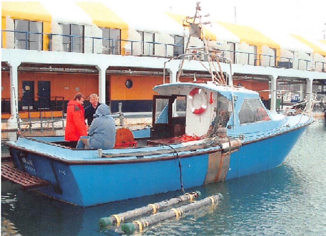
Figure 13 Survey Boat "Nikaria" With Sub-Bottom Profiler in Foreground
