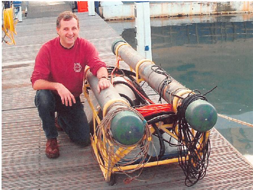
Figure 15 The Sub-Bottom Profiler Transmit / Receiver Tow Fish
