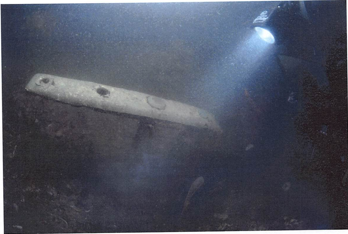
Figure 36. Rudder pintle on the 19 th century wooden sailing ship site. (copyright Michael Pitts)
