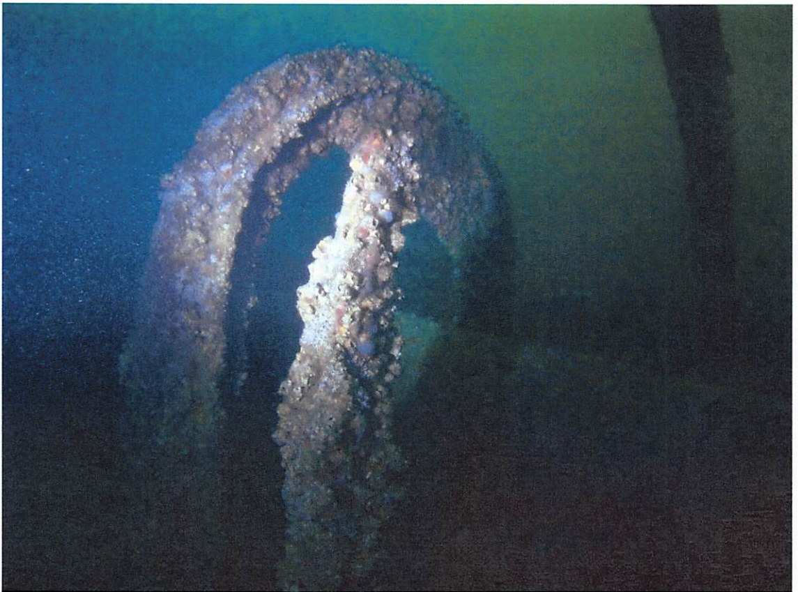
Figure 19. Propeller shaft and arch remaining from propeller tunnel. (copyright Dave Robbins)
